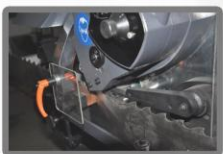
Precise stellite tipping long-lasting and minimum operation band saws providing perfect cutting surface quality.
