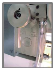
Cam-controlled tooth form swap
