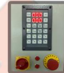
24V Control Panel
