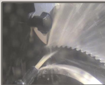
Automatic Right Chamfering
