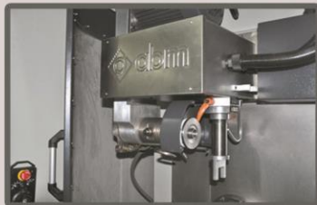
* Optional Laser Measuring System (Automatic diameter and number of teeth calculation)
