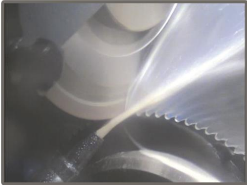
HSS Circular Saw Grinding by Ø200mm CBN Wheel
