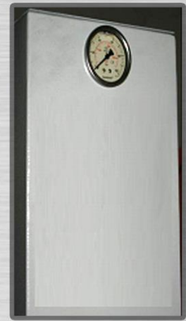
Hydraulic Tensioning Control by Hydraulic Gauge
