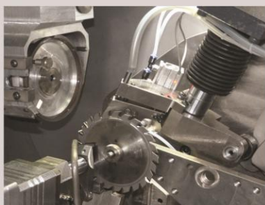
Automatic Broken teeth skip and Variable pitch indexing by intelligent finger. Optional pneumatic system for split (double-part) scoring blade grinding
