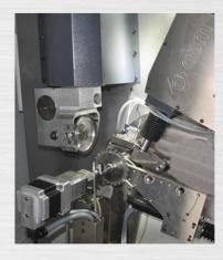
Automatic broken teeth skip and variable pitch indexing by intelligent finger. Optional pneumatic system for split scorer grinding in one pass.
