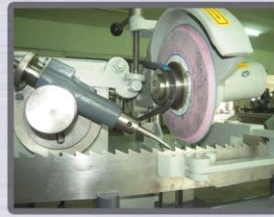
Fast grinding of band saws up to 100mm width.
