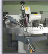
Rigid band saw holding.
